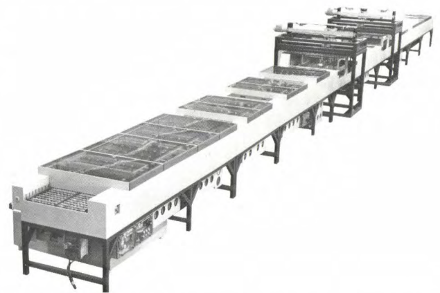
Fig. 11. Photograph of the machine for electroless silver deposition. This machine incorporates two metallization stations.
