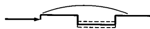
Fig. 16. Because of the slower rate at which the surplus charge flows back, the charge distribution at any particular instant is as shown here (and not as in the idealized representation in fig. 15c). The fraction of the charge left behind will flow to the right into the potential well that is forming and will introduce error by combining with the signal sample.
