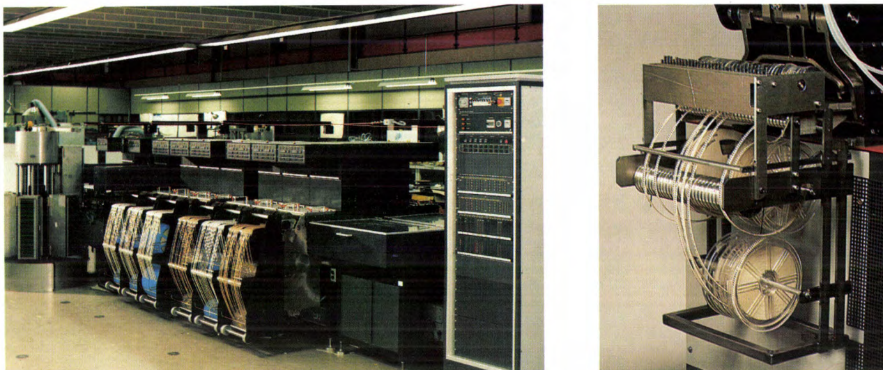
Fig. 4. Philips placing machine for multiple assembly of taped leadless components. The board feed, the application of adhesive to the boards, the transfer of components from tape to boards and the transport and removal of the assembled boards are all automatic. The machine has a capacity of about 250 000 components per hour. Right: Detail of tapes with components.
