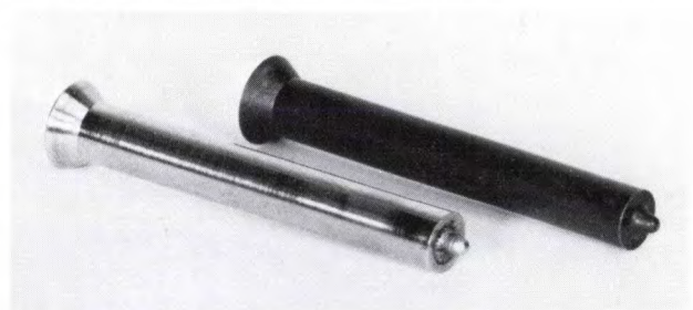
Fig. 10. Photograph ( 1.5 \times full size) of an uncoated riveting tool (left) and a riveting tool with a coating of 5 \mu\text{m} of TiC formed by CVD (right).
