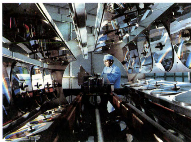
Fig. 9. Photograph of the evaporation area (above) and a carousel holder (below) for the deposition of aluminium on LaserVision discs.
