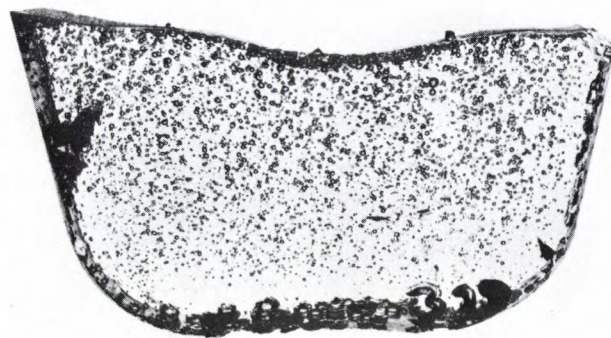
Fig. 1. Photograph of a cross-section of a glass melt that has been heated to 1450 °C and then rapidly cooled to room temperature. The bubbles to be seen consist mainly of CO 2 . To remove such bubbles rapidly, small quantities of a fining agent are added to the ingredients of the melt. The purpose of the research described here was to discover the mechanism of the fining process.
