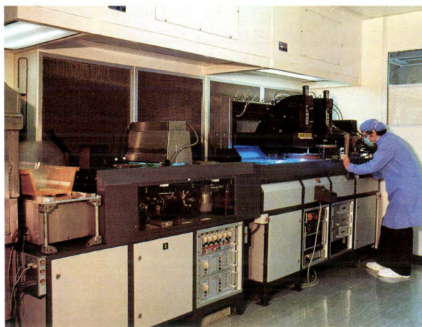
Fig. 7. General view of the 2p machine and related equipment. The machine on the right applies the 2p lacquer in manufacturing the LaserVision discs. The equipment on the left includes a post-exposure unit and a mechanical device for transferring the discs with cured lacquer to a holder.
