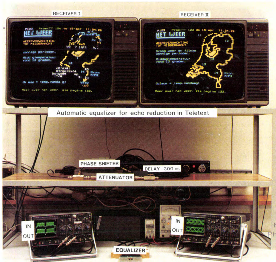
Fig. 4. Correction of the Teletext information by the equalizer. Receiver I : Teletext page degraded by the echo in fig. 3 . Many graphic elements of the test picture have been replaced by random alphanumeric characters. Receiver II : The Teletext page corrected by the equalizer. The oscillograms on the left show the time signals before and after the equalizer; those on the right show the eye patterns.
