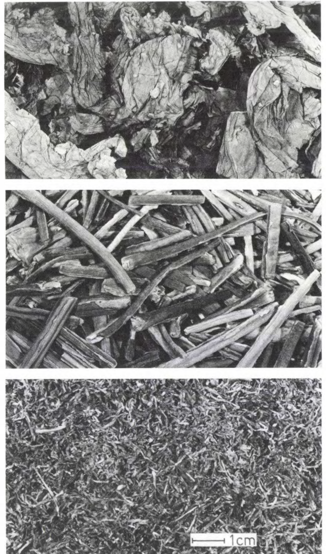
Fig. 15. Different structures in tobacco samples. From top to bottom can be seen successively leaves, stalks and the cut finished product. Moisture measurement in the tobacco industry should be affected as little as possible by these different structures.
